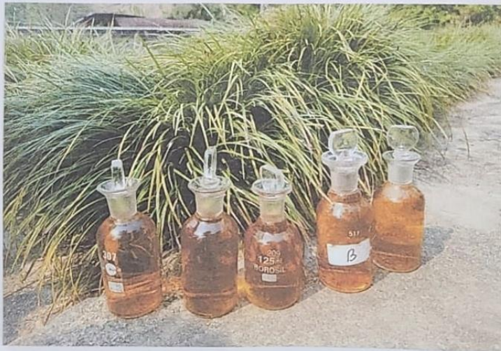
FIG: BOD BOTTLES AFTER ADDING KI, MnSO_4 AND CONC. H_2SO_4
